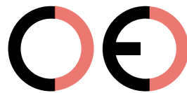
False CE Mark (too far)
